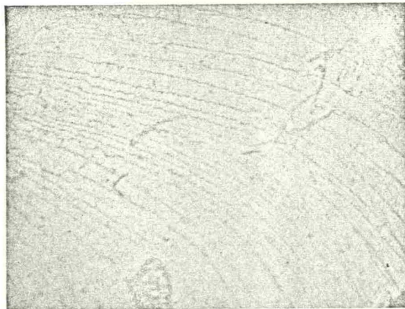
FIG. 2. Photograph of RbI crystal at a very early stage of its transformation to the high pressure phase. The near face of the crystal is in clear focus. Note the steps in the cleaved surface, the transformed "island" of surface on the back face of the crystal at the bottom of the photograph, and the island on the near surface at the upper right.
